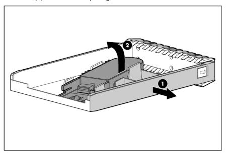
10. Position the replacement battery pack in the opening in the battery case as shown. The upper left edge of the battery pack is under the flanges on the pillars at the left edge of the opening, and the right side of the battery pack rests on the right pillars.
