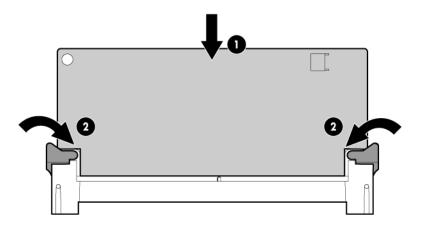
Install the capacitor pack onto the bracket, leaving sufficient room to connect the capacitor pack cable.
