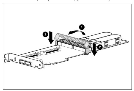
Reinstall the controller in the server.
