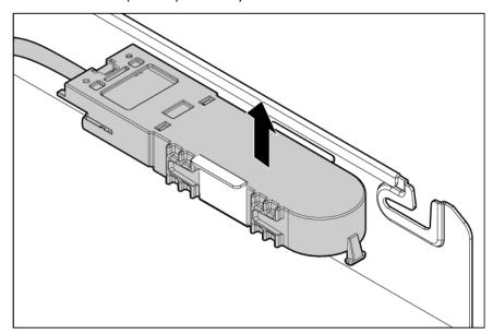
b. Disconnect the capacitor pack cable from the cache module.
