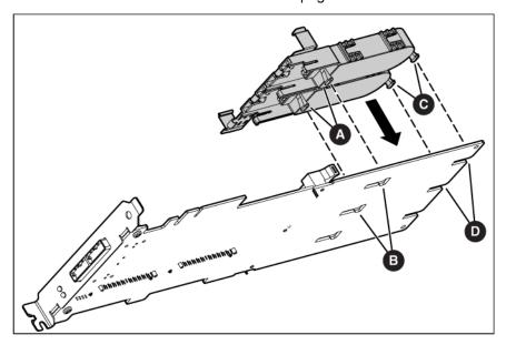
c. Slide the batteries toward the board bracket until they are firmly seated against the connectors on the cache module.
