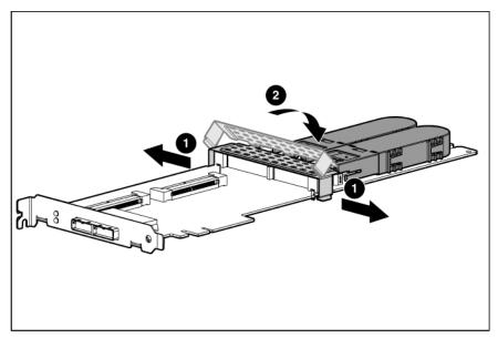
5. Slide the batteries toward the right edge of the controller, away from the bracket. While holding the battery assembly, tilt the clip until it is at about 30 degrees to the batteries, and then push the clip in line with the clip hinges until the clip detaches from the batteries.
