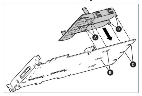
c. Slide the batteries toward the board bracket until the connectors on the cache module are firmly seated in the DIMM connector. (When the cache module is correctly seated, the gold contacts on the cache module are completely hidden within the DIMM connector.)
