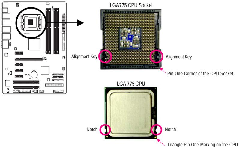
B. Follow the steps below to correctly install the CPU into the motherboard CPU socket.
