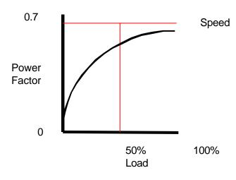
Figure 2. Induction Motor Power Factor
