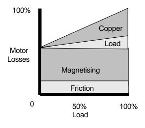
Figure 1. Induction Motor Losses
