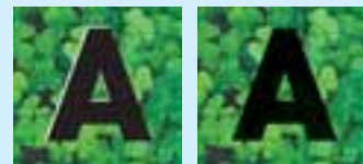
Overprint off Overprint on Black overprint ensures sharp text without white outlines caused by image creep
